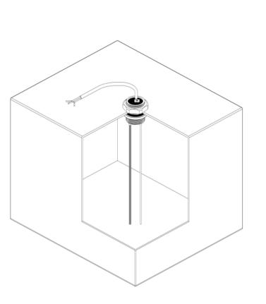
For remote level measurement, the **tank electrode** is installed directly at the tank. It is suitable for:
